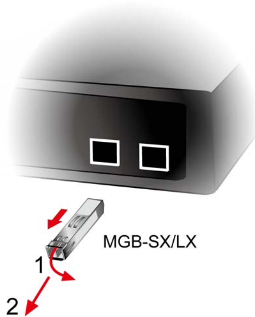
Figure 2-2-5: How to Pull Out the SFP/SFP+ Transceiver
